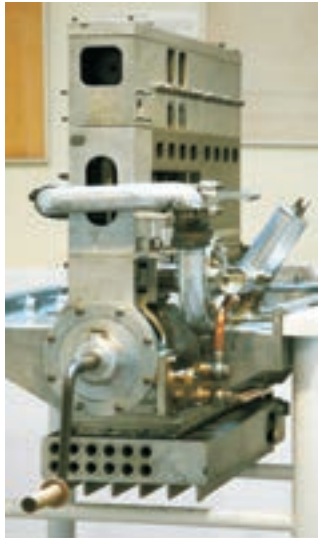
A 1930s poster which is part of the permanent exhibition and below, a sectioned Bugatti engine
